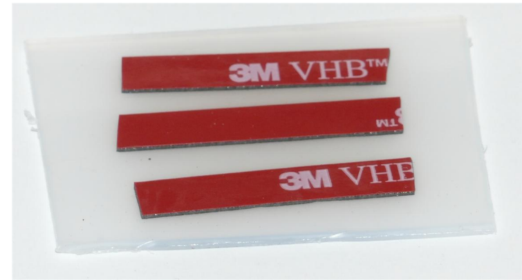
Tape to secure wires.
